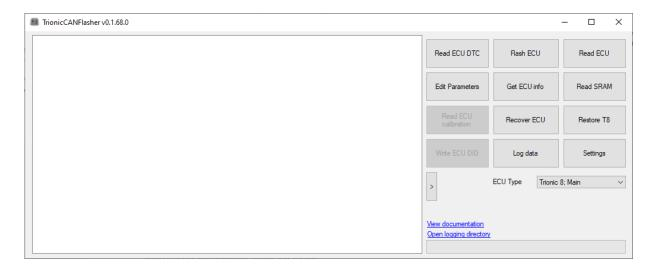
Now click on "Settings", under "Adapter type" select the "OBDLink SX". Under "Adapter" select the corresponding COM port.
