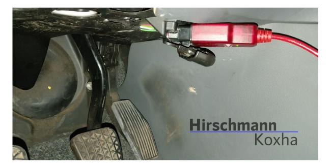
Now turn the ignition key to the "ON" position and switch off all stuff such as the radio, headlights, seat heating, air conditioning, etc.
