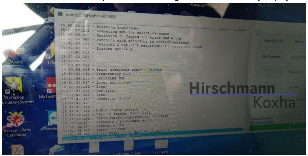
Pay close attention to the "MCP firmware information" and the "Version string" below. If your vehicle is not a facelift (model years up to 2006), you must have the MCP R1.0 on it. For vehicles of model year 2007 and newer, the MCP R1.1 is required.
